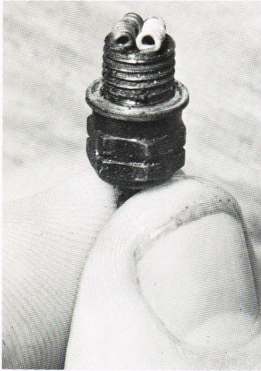
"Glow plug" used in the endurance flight. (All photos are by Fremont Davis.)
