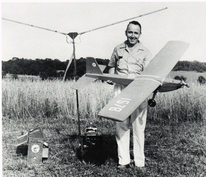
The author is shown with a modern radio-controlled model and its supporting ground equipment. This model has radio control of its rudder, elevator, ailerons, flaps, and engine.
