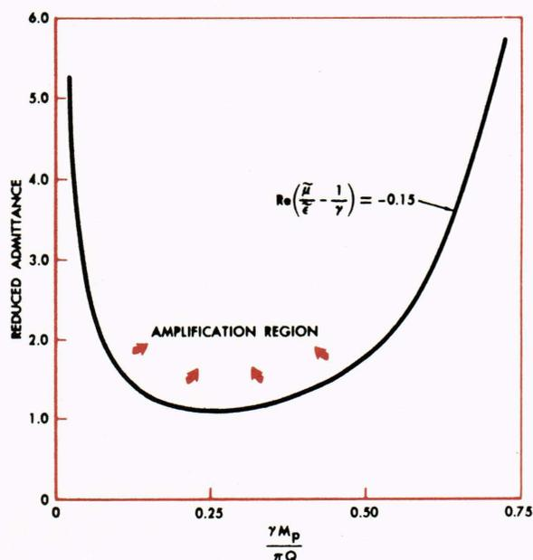
Fig. 12—The effect of finite amplitude and erosion on stability in axial modes for a hypothetical propellant. The ratio of acoustic pressure amplitude to the mean pressure is  $Q$ , and the port Mach number is  $M_p$ .
