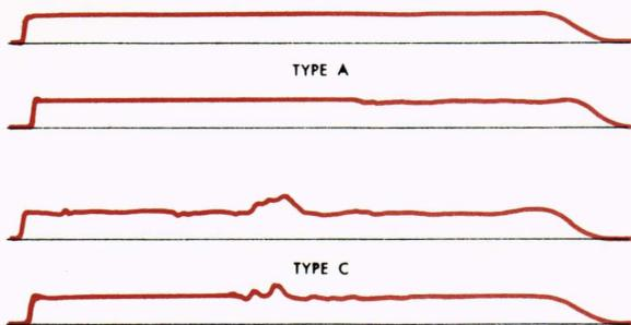
Fig. 6—The effect on stability of tightness of fit of the propellant grain is shown here by mean pressure traces at 70°F. Type A fit is the tight fit, and Type C is the controlled loose fit. (From T. Angelus.)
