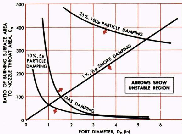
Fig. 9—Neutral stability contours corresponding to various kinds of damping mechanisms. The arrows point into the unstable region.
