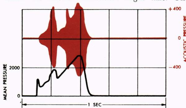
Fig. 2—Oscilloscope trace showing pressure. The upper trace is the oscillatory pressure component, and its magnitude is read off on the right-hand ordinate scale. The lower trace is the mean pressure, as indicated by the left-hand scale. (From E. W. Price.)
