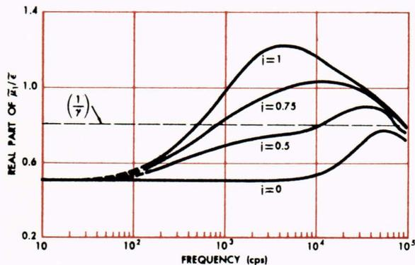
Fig. 5—Pressure response of four hypothetical propellants, each having a pressure index  $n = 1/2$ , but having four different temperature indices ( $j = 0, 1/2, 3/4, 1$ ).
