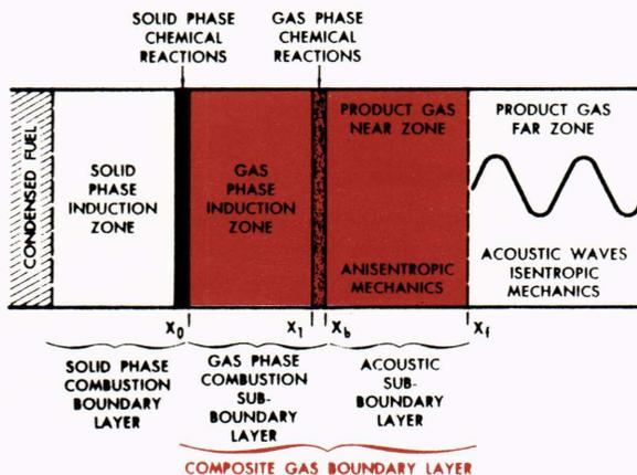
Fig. 10—Schematic representation of the gas-solid boundary region.
