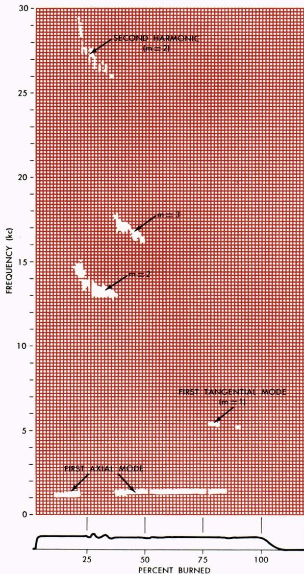
Fig. 3—Frequency versus percent of web burned, illustrating the usual occurrence of oscillations in acoustic modes and, for very large amplitude cases, in harmonics of the acoustic modes. (From T. Angelus.)
