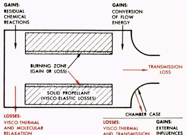
Fig. 8—Schematic representation of a rocket motor showing possible sources of acoustic gains and losses.
