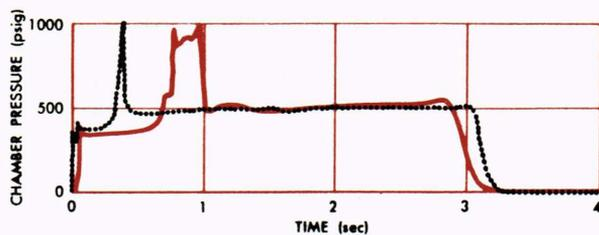
Fig. 1—Pressure-time traces characteristic of an unstable rocket motor. The two curves correspond to two firing temperatures. (From W. G. Brownlee.)
