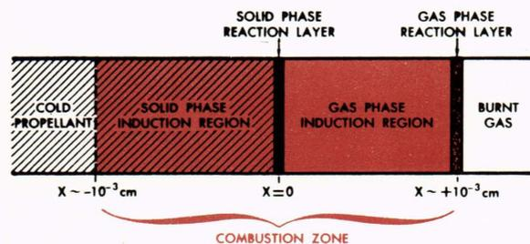
Fig. 4—Schematic illustration of the combustion region.
