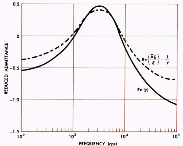
Fig. 11—The effect of entropy wave generation on amplification by the burning propellant. Amplification occurs above the X-axis.
