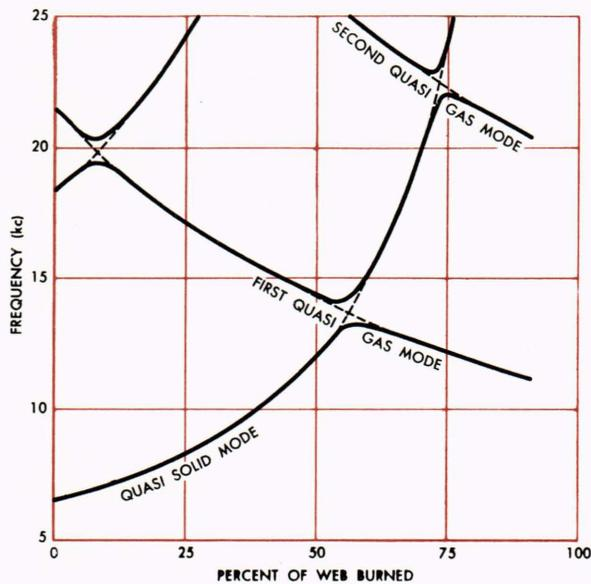
Fig. 7—Frequencies of the lowest transverse mode and its first two overtones for a cylindrical grain.
