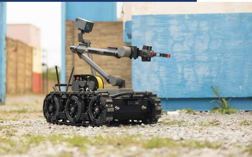
APL is advancing autonomy and sensing that help warfighters detect and mitigate explosive hazards using fielded robotic platforms such as the Man Transportable Robotic System Increment 2, shown here during an explosive ordnance disposal field exercise at Camp Hansen, Okinawa, Japan. Credit: U.S. Marine Corps
