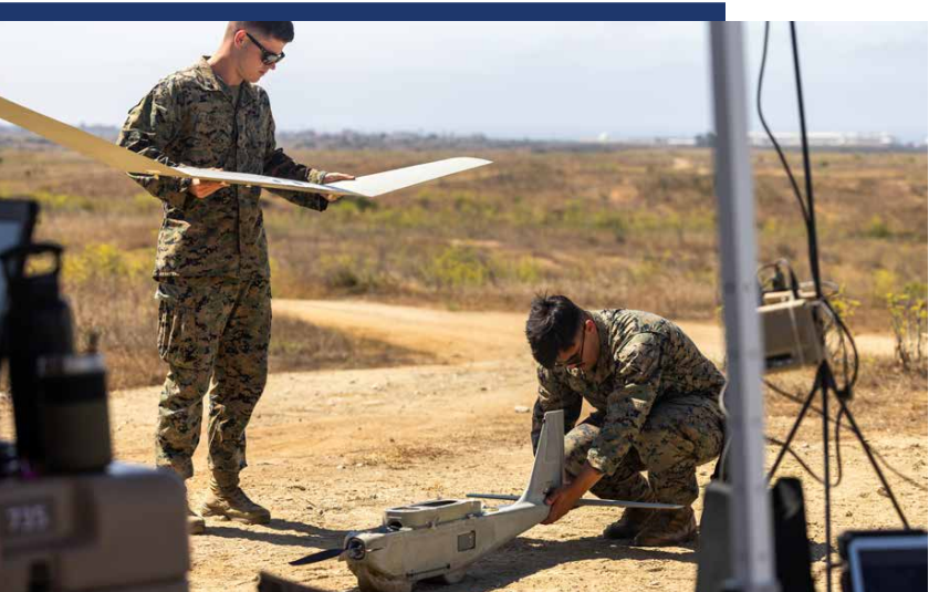
Dead Center is an APL-developed low-SWaP artificial intelligence system that performs real-time onboard target detection on autonomous platforms, sending only concise data to reduce bandwidth and enable fully autonomous intelligence, surveillance, and reconnaissance missions. Marines with 1st Light Armored Reconnaissance Battalion train with Dead Center at Camp Pendleton in August 2025. Credit: U.S. Marines Corps
