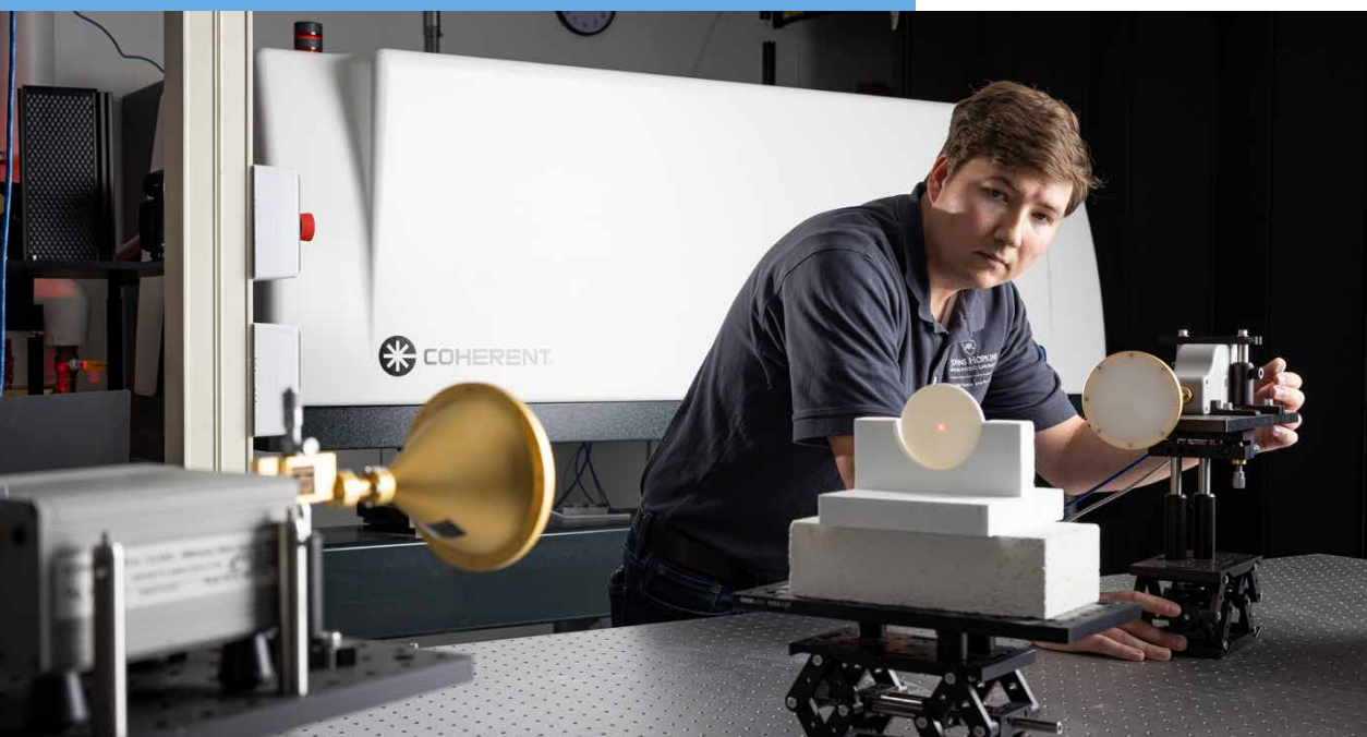
Andy Goers, an APL optical physicist, works in the Hypersonic Optical Test Lab. This facility is a versatile space where APL researchers use a high-power CO 2 laser, infrared pyrometry cameras, wavefront sensors, and a boresight-error testbed to evaluate and characterize advanced hypersonic materials and coating concepts.
