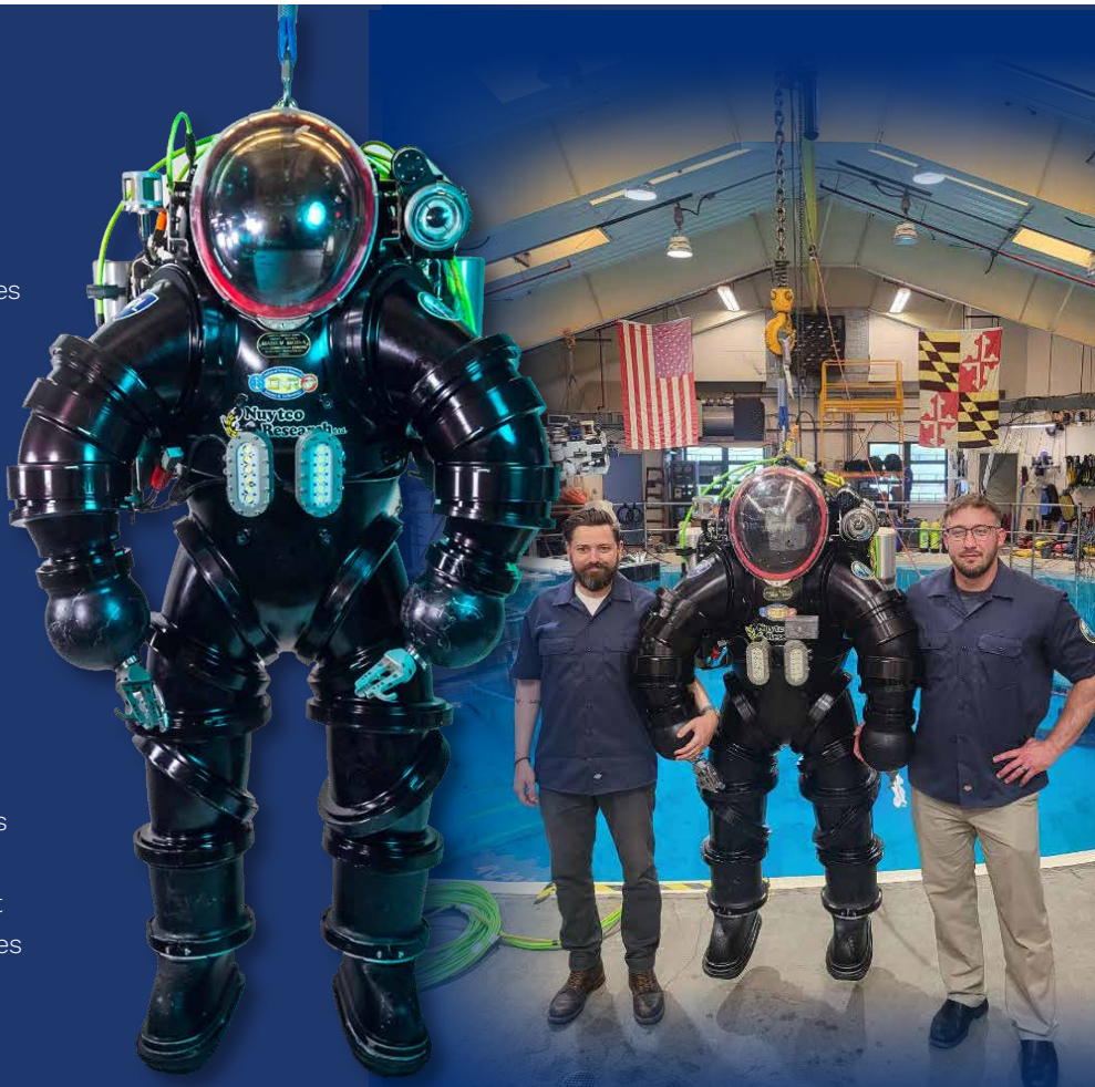
The Deep Sea Expeditionary No Decompression (DSEND) prototype atmospheric diving suit is shown above. The suit was tested in water at the U.S. Navy Experimental Diving Unit and demonstrated at the University of Maryland in June 2025 with APL project manager Chad Klinesteker (left) and program manager Alex Cheij. Credit: Charlie Hanner (DSEND image at left)
