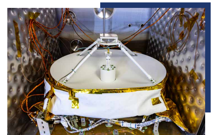
Hardware for PEXT undergoes environmental testing at APL, helping validate a wideband communications approach that can link spacecraft to both government and commercial networks.
