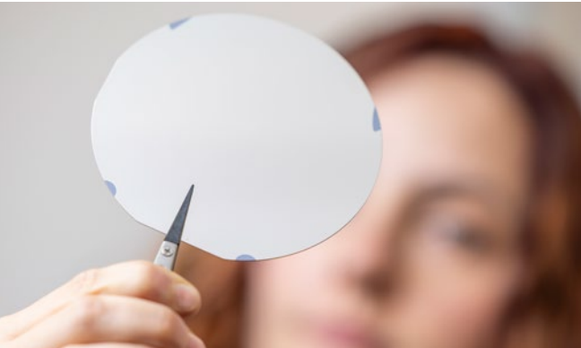
Materials scientist Bella Hunt holds a wafer with a novel thermal coating technology developed at APL that enables advanced materials to efficiently manage thermal conditions in buildings and data centers.
