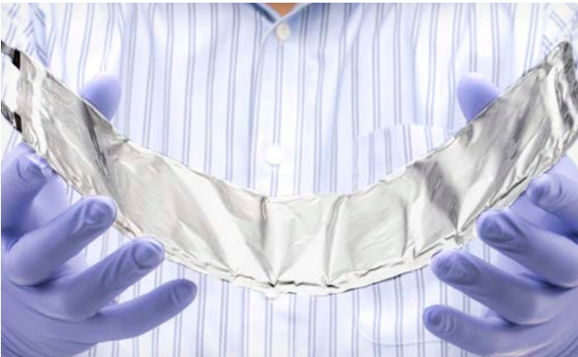
APL researchers synthesized aluminum niobate from scratch using a method that could be replicated at commercial scale, and demonstrated operation in pouch cells (seen here)—one of the main types of commercial batteries—with high energy.
