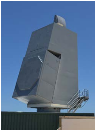
The AN/SPY-6 Air and Missile Defense Radar array (right) installed on the USS Jack H. Lucas (left), the latest destroyer in the Arleigh Burke class, is the first of four SPY-6 designs in development. (Credit, from left: U.S. Navy and Raytheon)
