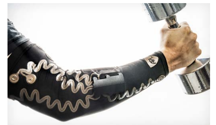
Using a stretch athletic textile developed at APL, EXOForce Robotics is creating intelligent garments that can sense muscle behaviors and whole-body biomechanics, and use machine learning to tailor readouts to the wearer, quantify their workouts and alert them to impending injury.
