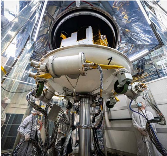
APL engineers move the Double Asteroid Redirection Test (DART) spacecraft into a thermal vacuum chamber, where it was subjected to the extreme temperatures and other conditions it will face in space.
